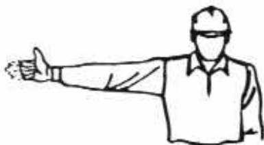
LOWER THE LOAD RAISE THE BOOM
