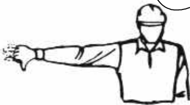
RAISE THE LOAD LOWER THE BOOM
